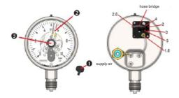
The set points are adjusted from the outside via an adjusting lock in the window.
