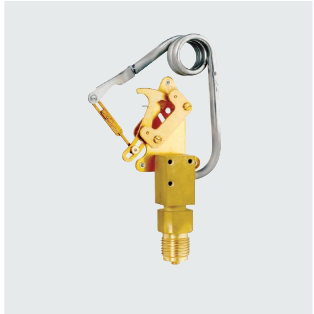
Bourdon Tube Measuring System, Helical Form
